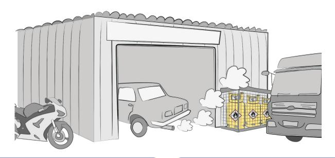
If vehicles have to be run, minimise the running time and connect the vehicle's exhaust to extraction equipment.
