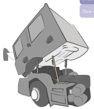
When you work on raised tipping trailers or vehicle cabs you should ensure that additional supports are in position to prevent the trailer or cab descending and crushing workers. This is because the rams to lift the loads cannot be guaranteed to keep the load raised while workers are underneath.
